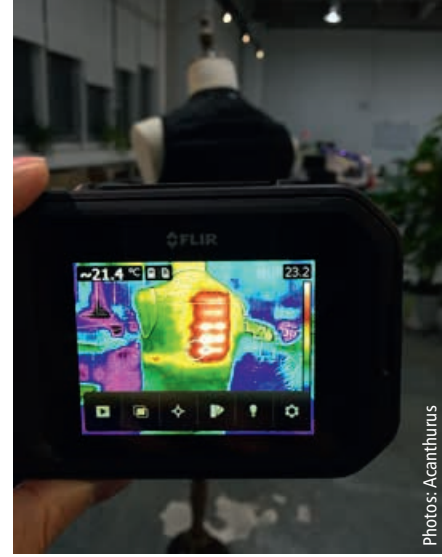
J-Nova is a collection of groundbreaking thermal conductive textiles and fibers, which are able to conduct and store heat without any wires or cables
