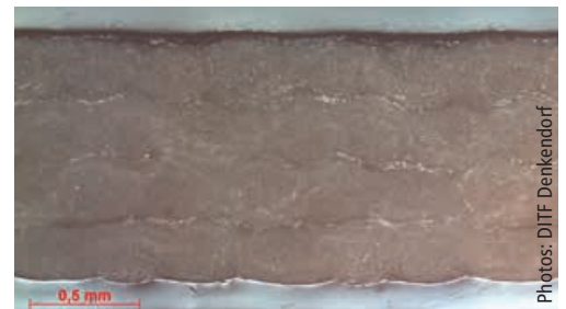
Purcell composite plate (cross-section), comprising 4 layers
