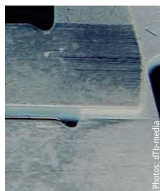
Tempestini, Italy shows the lower wear with the comparison patterns – Nano-technology (bottom)
