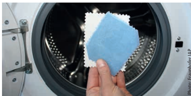
Even after multiple washings, the textile retains its color due to the blue microcapsules. This shows how stable the capsules are and how well they are affixed to the textile
