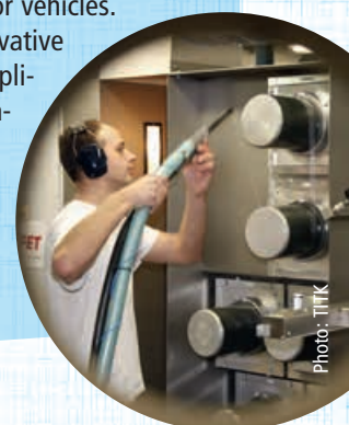
Bioplastic as a matrix polymer for switchable yarns: TITK employee with multifilament strand at a melt-spinning system
